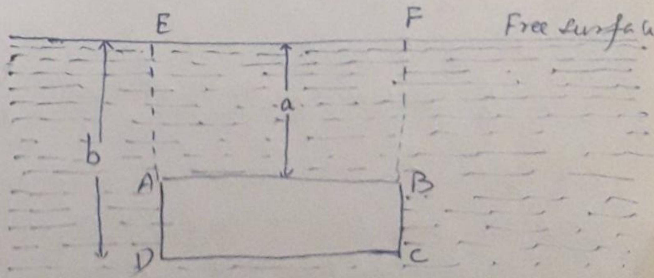
The thrust on the rectangle  $EFCD = \rho g \cdot \frac{b}{2} \cdot hb = T_1$  (say),
