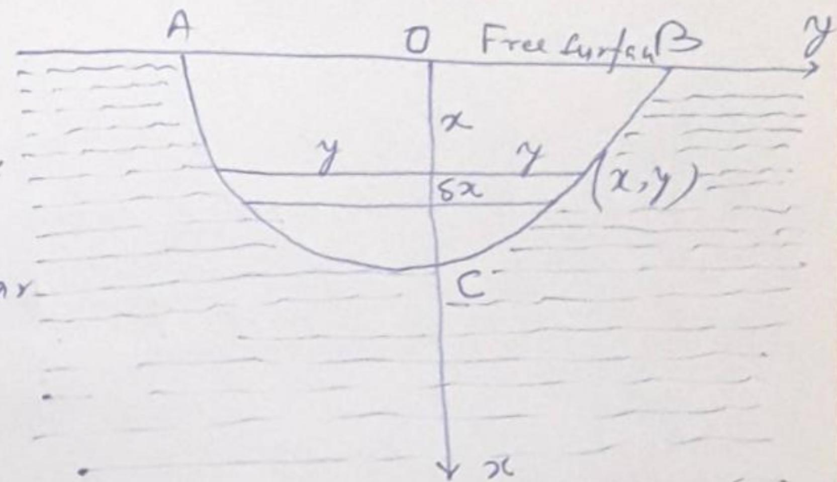
Ex-7 An ellipse is just immersed with its major axis vertical. Show that if C.P coincides with the lower focus, the eccentricity of the ellipse is  $\frac{1}{4}$ .
