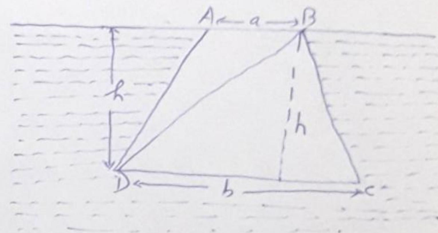
$$\text{Also the thrust on } \triangle BCD = \rho g \cdot \frac{2h}{3} \cdot \frac{1}{2} bh = T_2 \text{ (say).}$$
