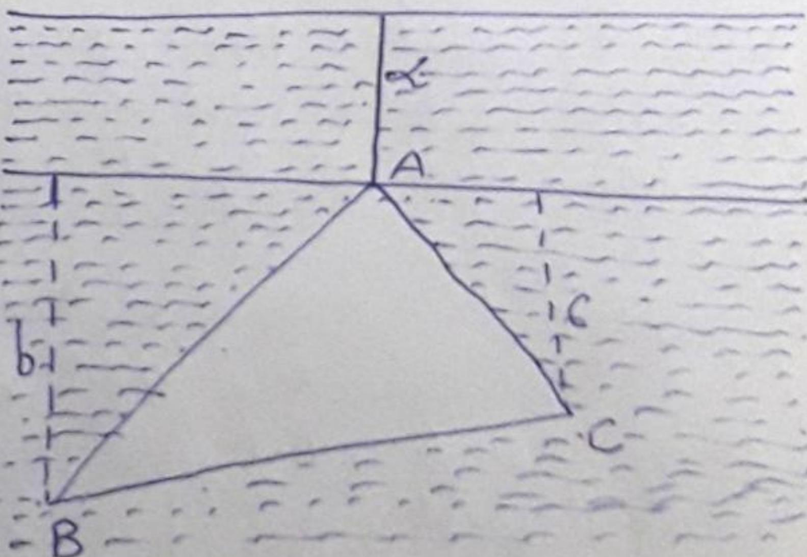
On account of the lowering of the triangle through a depth  $\lambda$ , there will be an additional thrust,  $T_3 = W \Delta \lambda$ , acting at the C.G. of the triangle whose depth below the horizontal through A is  $z_3 = (b+c)/3$
